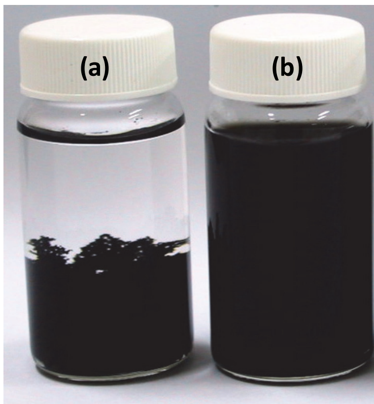
Fig. 4. Optical micrographs of MWCNTs dispersions in water in the presence of SDS surfactants prepared by means of (a) a bath sonication process for 8 h and (b) a high-energy probe type sonication process for 3 min, respectively.
