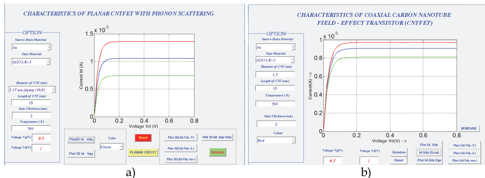
Fig. 19. The diameter dependence of I_{DS} - V_{DS} characteristics at V_{GS} = 0.7 V in CNTFET having the length of 15 nm under scattering: a) in planar CNTFET ON-current increase by 8, 11, 14 \mu A when diameters of CNT increase by 1.25, 1.5, 1.7 nm, respectively, b) in coaxial CNTFET under scattering, ON-currents increase by 8.0, 9.0, 9.5 \mu A when diameters of CNT increase by 1.25, 1.5, 1.7 nm, respectively.
